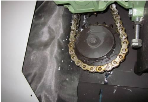
Lager schmieren (Mobilux EP 2/NLGI 2)
