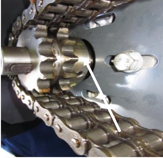
Lager schmieren (Mobilux EP 2/NLGI 2)
